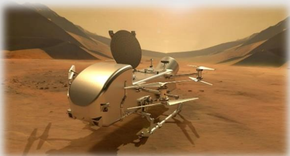
Artist's impression of the Dragonfly rotorcraft lander on the surface of Titan. (Image credit: NASA/Johns Hopkins APL/Steve Gribben)
